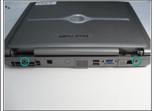
15-1. Remove ~~1ea M2.5 x 8mm~~the screw holding the EMI shield in place.
