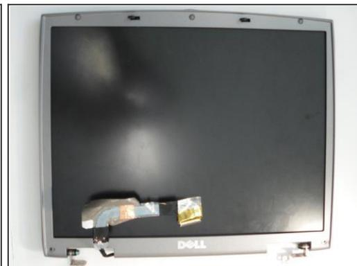
**Warning:** Open the lid and support the display assembly while performing the next step to prevent the display assembly from falling down when you remove the hinge screws.
